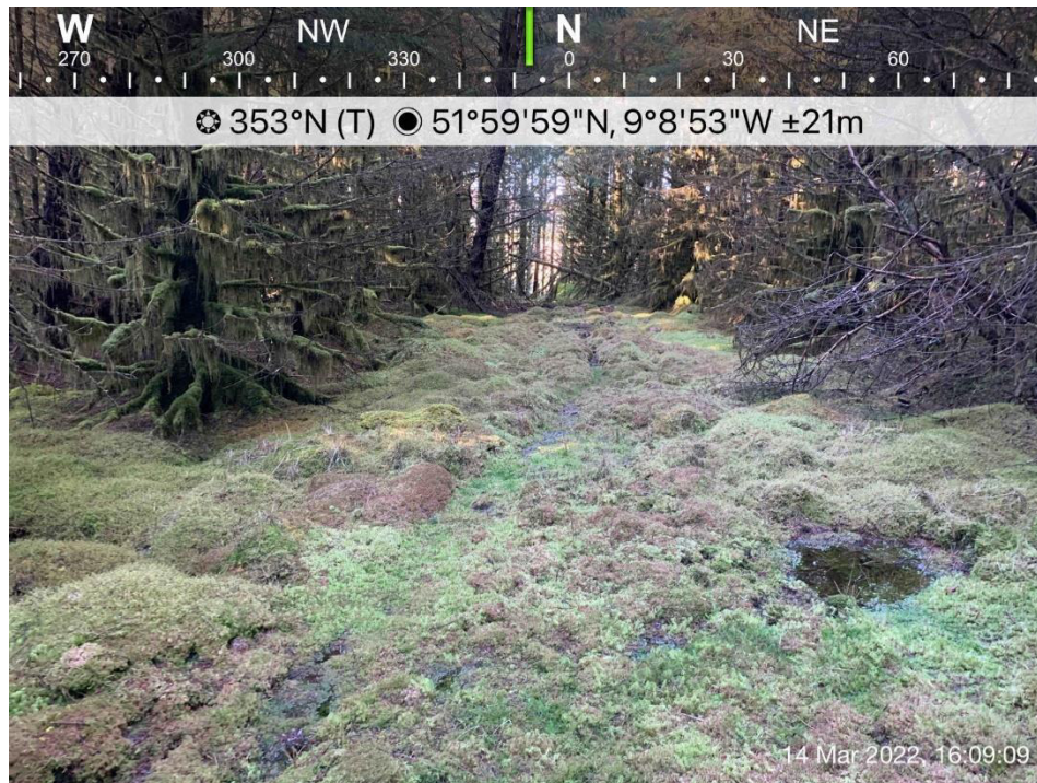
Figure 2-4: Area of wet, saturated peat material in topographical low area adjacent to a steep topographic shoulder north of T4
